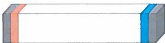
Figure 11. Simulation box including fixed slabs (gray), 350 K slab (red), 250 K slab (blue), and middle slabs (white). [Color figure can be viewed at wileyonlinelibrary.com ]
