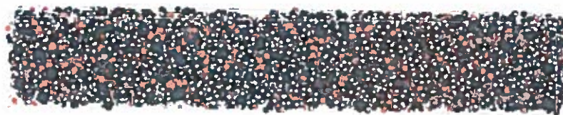
Figure 10. A representative prism-shaped model for determining the thermal conductivity using NEMD. [Color figure can be viewed at wileyonlinelibrary.com ]
