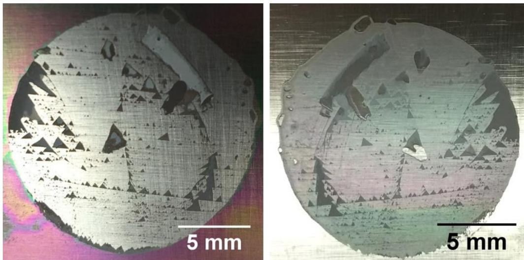
**Fig. 4. Typical surfaces from nanotube shear tests. (Left) Pink-green area outside the central circular region are nanotubes not involved in the test. The circular bright area is the titanium after the nanotubes were sheared away. The dark areas are failed adhesive. (Right) Corresponding surface showing faint pink-green hue within circular region indicating bottom of nanotubes pulled from the shiny region at left.**
