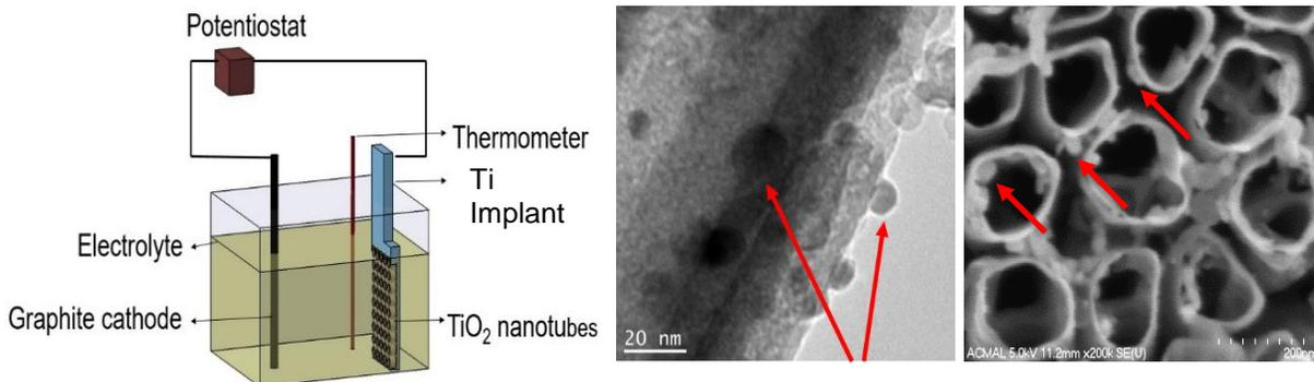
**Fig. 1. Simple DC anodization with non-hazardous electrolyte etches surface leaving nanotubes, in as little as 10 minutes. Very small addition of silver compound (patented) produces nanosilver spheres decorating nanotubes in same process.**
