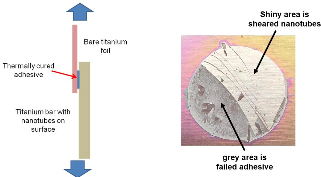
**Fig. 3. (Left) General arrangement for conducting shear strength tests of nanotube surfaces. (Right) Typical surface after specimen test. The circular region is 0.6-inches diameter and required 1,523 pounds (6.78kN) of shear force to cause failure.**
