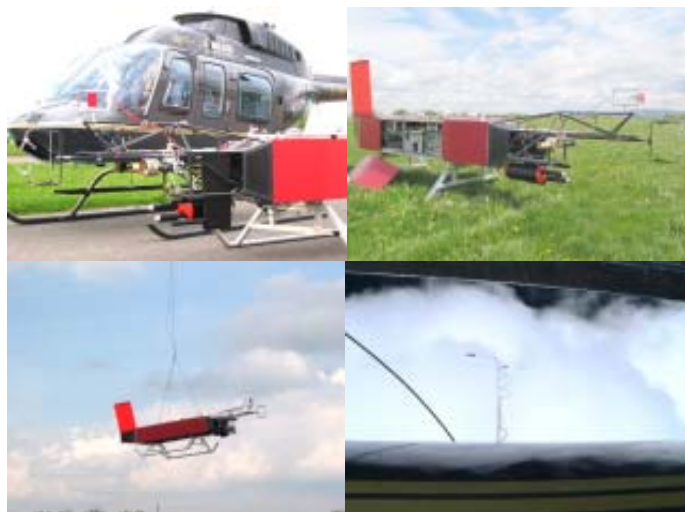
Clockwise: Helicopter; instrument payload: ACTOS; view from the helicopter, looking down on ACTOS, in the clouds; ACTOS takeoff.
