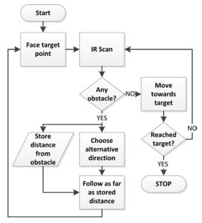
Fig. 7. Path planning and target reaching algorithm
