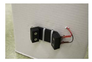
Fig. 2. Female magnetic connector 2.2 Power Source and Power Load Connections
