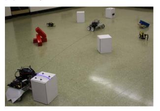
Fig. 12. Agent has autonomously connected the power source to the power load
