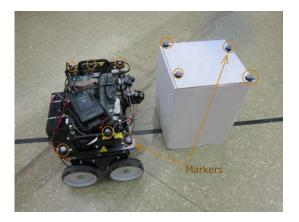
Fig. 3. Marker placement on robot and object
