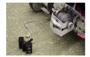
Fig. 1. Male magnetic connector with wire pulley
