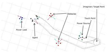
Fig. 10. Test results of agent avoiding obstacles and reaching the touch point of power source (agent is positioned at the start point)
