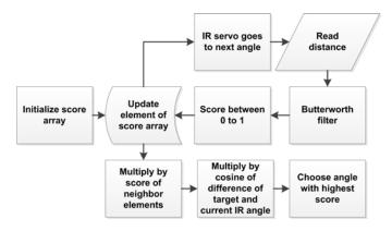
Fig. 8. Direction choosing algorithm using IR scan
