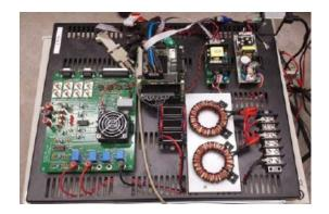
Fig. 13. Power Electronic Building Block (PEBB)
