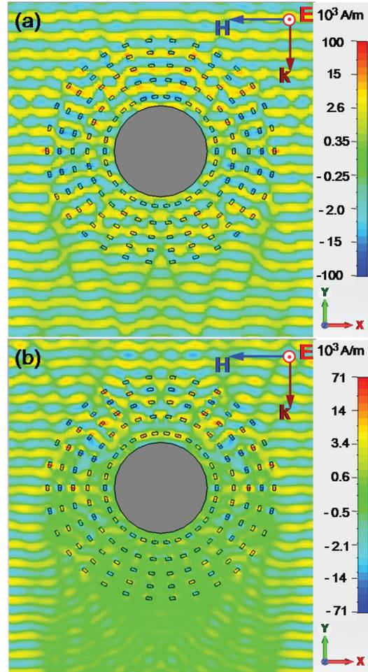
FIG. 4. (Color online) Simulation of TE plane wave incidence on an infinite five layered cloak of  $4\ \mu\text{m}$  thickness concealing a metallic object of  $5\ \mu\text{m}$  in diameter. The effective permeability values of the first to fifth layers are 0; 0.056; 0.134; 0.2; and 0.257, respectively. Corresponding radii of these layers are 3000, 3925, 4720, 5430, and 6095 nm. Cloaking at 286.3 THz (a) and shadow at 297.1 GHz (b).
