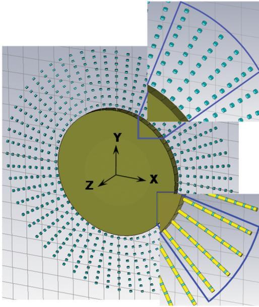
FIG. 3. (Color online) A glass cloak designed to hide a metal cylinder of  $15\ \mu\text{m}$  in diameter; upper inset highlights different distances between the resonator arrays; and lower inset depicts cylindrical spokes comprising glass resonators and fused silica spacers.
