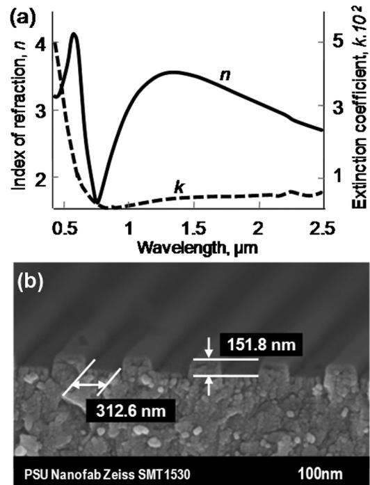
FIG. 1. Spectral behavior of refractive index and extinction coefficient of a GeSbSe thin film (a) and a GeSbSe grating structure fabricated by using e-beam patterning (b).
