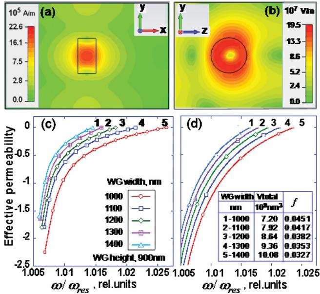
FIG. 2. (Color online) Halos of magnetic (a) and electric (b) fields around cylindrical glass resonator, and frequency dependencies of  $\mu_r^{\text{eff}}$  extracted from simulated scattering parameter spectra for single-resonator unit cells of different widths (c), and analytically calculated for these cells with  $V_{\text{halo}} = 0.35 \times 10^8 \text{ nm}^3$  (d).
