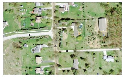
Figure 3-44: Example of RGB aerial photography being analyzed with image processing to map the location of unpaved vs. paved roads in SE Michigan as a mission planning input.
