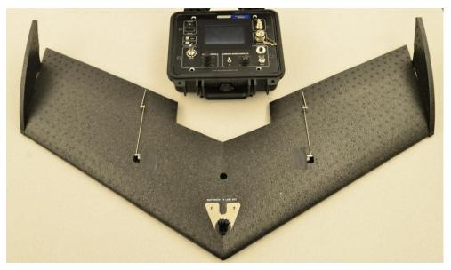
Figure 3-2: Lehman LP-960 wing and ground control station.
