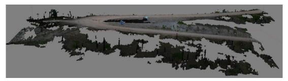
Figure 3-23: 3D point cloud of the Stratobowl collect after the trees were removed from the model.
