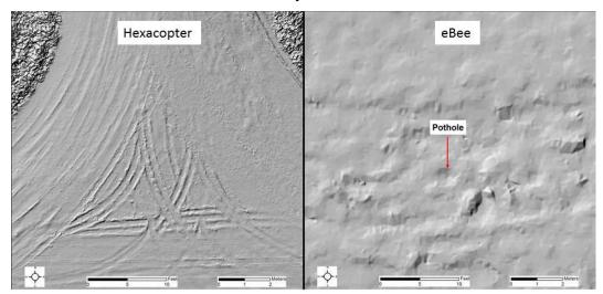
Figure 3-7: A comparison between the level of detail between DEMs generated from the Bergen hexacopter-based system and an eBee-based data collection system. Both hillshade representations are at the same scale and the pothole pointed out in the eBee hillshade is 67cm in width.
