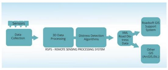
Figure 2-1: The flexible, modular components of AURA developed as a working prototype for this project.
