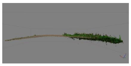
Figure 3-15: 3D point cloud on a section of unpaved road from the demonstration site illustrating the project team's capability to make crown measurements.
