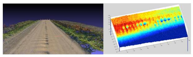
Figure 2-4: A 3-D point cloud generated through the project's algorithms and the corresponding height map where potholes and their depths can be seen.
