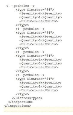
Figure 3-32: An example of the XML output from RSPS run on the Piotter Highway point cloud and categorizing detected potholes into severity categories. For example, one high-severity ("H") pothole was detected in this stretch.
