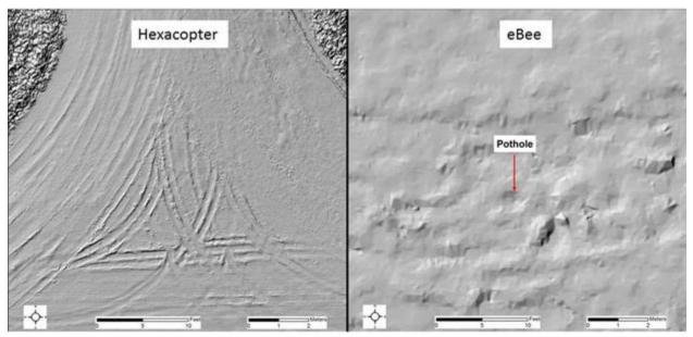
Figure 1-1: A comparison between the level of detail between DEMs generated from the Bergen hexacopter-based system and an eBee-based data collection system. Both hillshade representations are at the same scale and the pothole pointed out in the eBee hillshade is 67cm in width.
