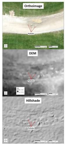
Figure 3-6: Detail of potholes on an unpaved road in Shelburne, VT. The orthoimage and DEM were generated in Pix4D and the hillshade was generated in ArcGIS from the DEM. Both the orthoimage and DEM are processed to a resolution of 3.3cm.
