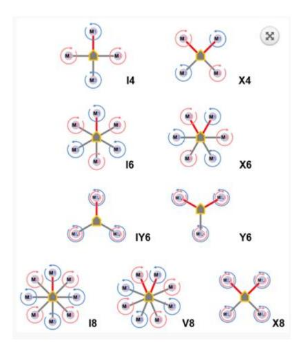
Figure 3-1: Possible multi-rotor prop configurations.
