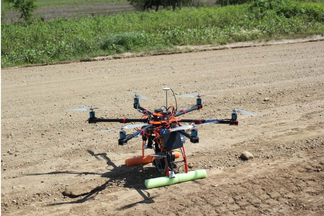
Figure 7-2: Existing hexacopter system from Bergen used to evaluate unpaved road condition in 2013 and 2014.
