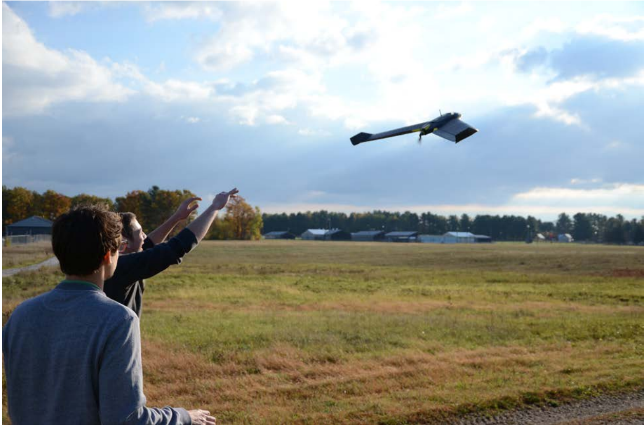
Figure 2-6: Hand launching of an eBee (Photo Courtesy of Jarlath O'Neil-Dunne)
