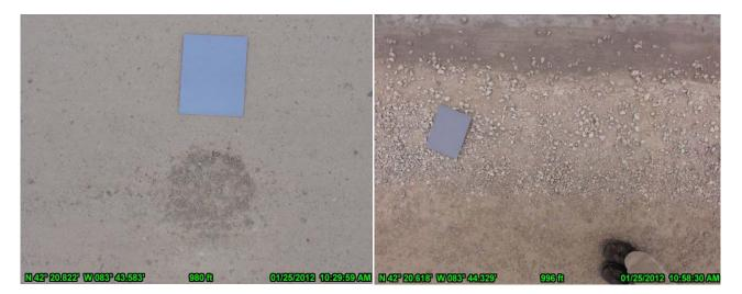
Figure 1: Example of how lighting and camera effects can change the measured color of a scene.
