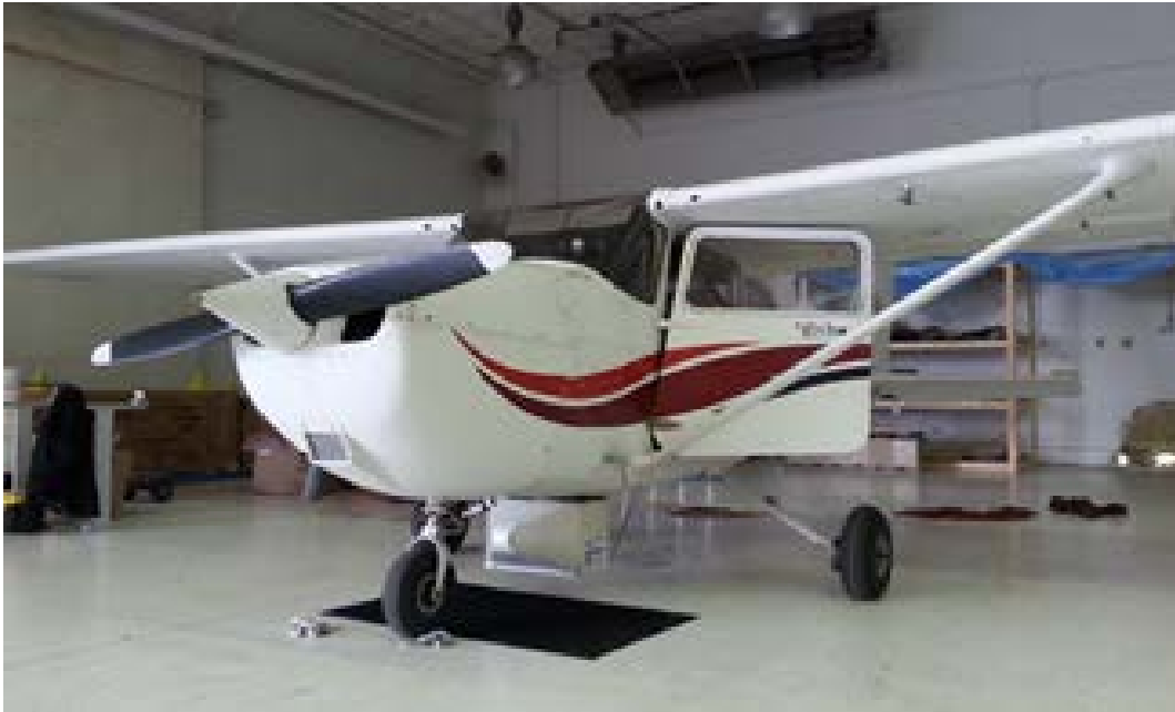
Figure 5: Surrogate Unmanned Aerial System with sensors mounted below the aircraft's fuselage.
