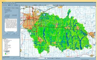
Figure 1: The WMSST tool has been used to create an analysis of suitability for potential wetlands mitigation for an entire 294,000 acre watershed. The tool is docked on the left within an ArcGIS interface; blue areas have the highest suitability.
