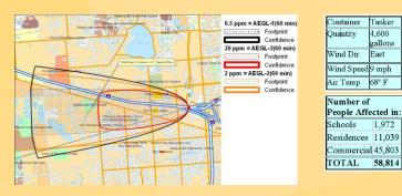
Figure 3: Demonstration of an integrated toolset that analyses the impact of a highway-based chlorine spill on the surrounding local area. The TARUT Study analysis made possible calculations of number of people and businesses affected in addition to the traffic volumes and amount of roads impacted by the plume.
