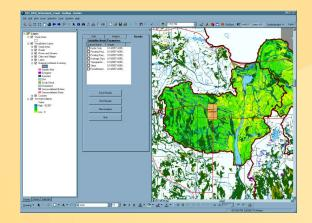
Figure 4: The Wetlands Mitigation Site Suitability Tool has been used to evaluate 76,000 acres for locatiing the best areas for constructing wetlands mitigation sites. The blue and darker green areas are the most suitable based on soils data, remote sensing-based soil moisture analysis, topography, and historical wetland status.
