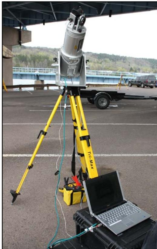
**Figure 18: Typical Reigl LiDAR unit setup.**
