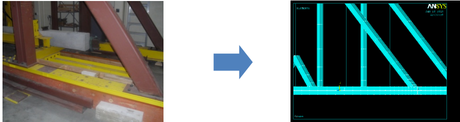
Figure 1b. Close up of meshing capability in finite element model compared to digital photo image
