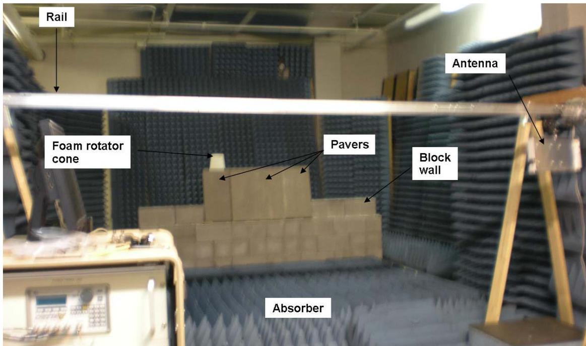
**Figure 1d: MTRI antenna chamber with Lab Genie set up.**
