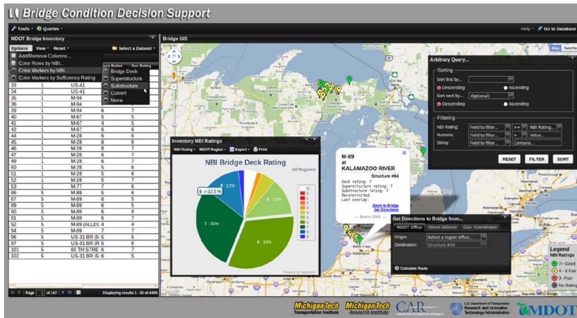
Figure 1: An example screenshot of the current Quarter 6 version of the Bridge Condition Decision Support System. Note the availability and integration of data from MDOT's Bridge Management System with querying and display tools; integration of remote sensing results is planned next due to the upcoming field demonstrations.
