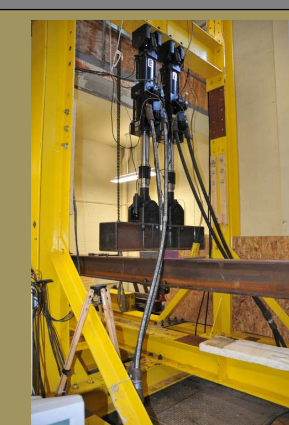
Digital Image Correlation Experiment: Steel beam mounted to be deflected
