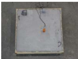
Specimen with simulated defects
