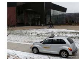
Michigan Tech's LiDAR mobile mapping system & Rozsa building point cloud
