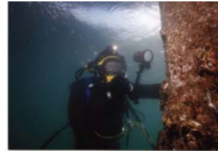
Camera device used in underwater inspections Fig. 11.3.47 Bridge Inspection Reference Manual (2005).
