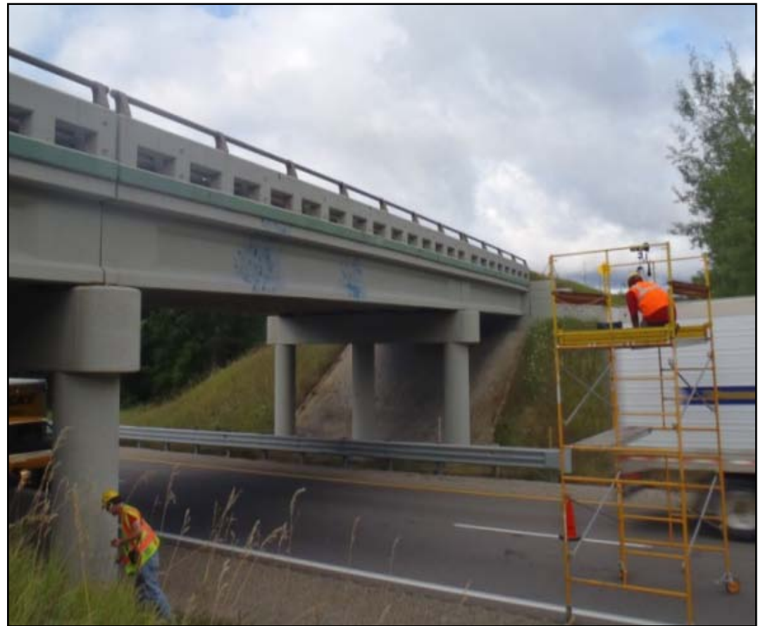
Scaffolding setup at Mannsiding Rd. bridge facing exterior girder with speckle patterns
