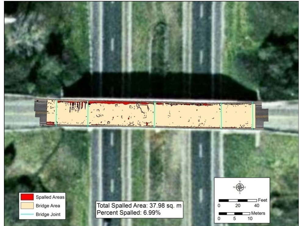
Visual of percent spalled area for the Willow (6.99% spalled) Road bridge using 3DOBS data as the input and ArcGIS as the analysis software
