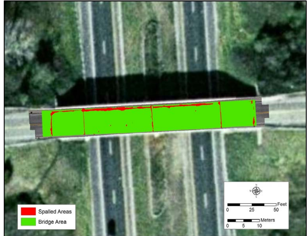
Visual of percent spalled area for the Willow (6.08% spalled) Road bridge using 3DOBS data as the input and ArcGIS as the analysis software
