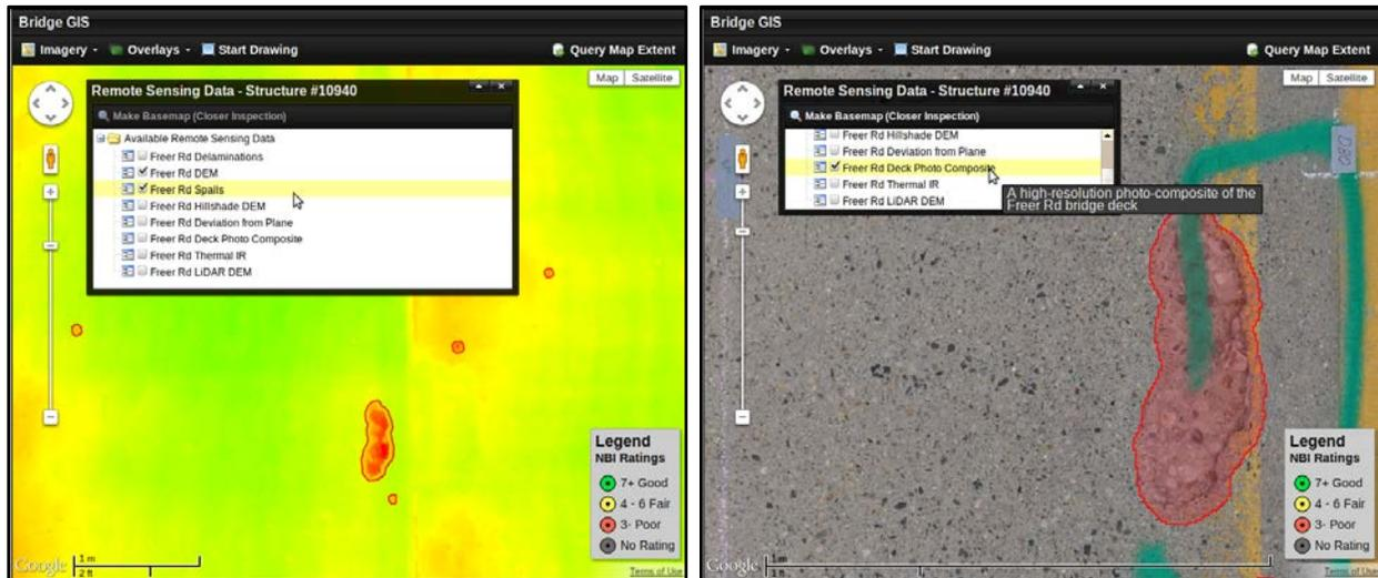
**Figure 13-9:** Screenshot from DSS of a digital elevation model (DEM) with a color-ramp and spalls outlined in red (left) and screenshot of a high-resolution photo composite showing the same, large spall as outline on the left; note the scale bar at the bottom of each, which is 1 meter in both (right).
