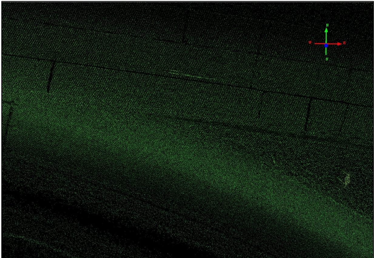
**Figure 7-25: Close up of the LiDAR return pattern where a ramp where data was collected at 35 mph meets the main road where data was collected at 45 mph. The distance between scan lines increases with vehicle speed. The ramp diverges from the main road to the lower right in this image. Elevation and intensity values are displayed in this image.**
