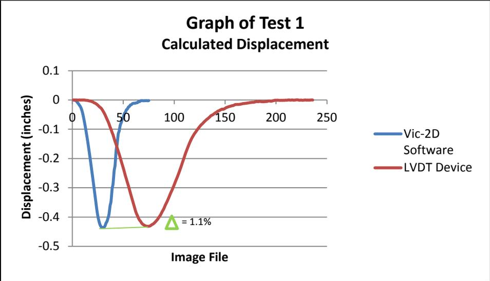
Figure 9-10: Graph of LVDT Result and DIC measurements.
