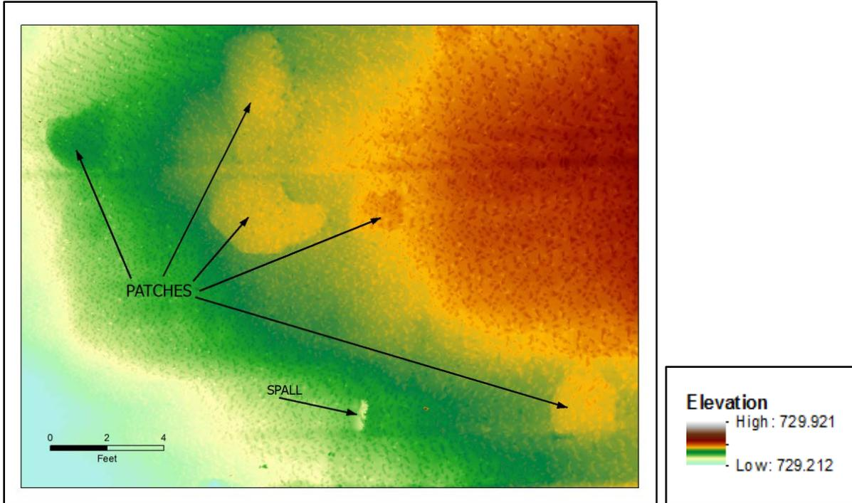
**Figure 7-21: DEM with a color ramp applied of the same area of the Willow Road bridge deck. Note that the higher areas of the concrete patches and missing material from the spall correlate well between the ortho-photo and DEM. The patches (correctly) appear higher than the surrounding bridge deck and the spall appears lower than surrounding deck.**
