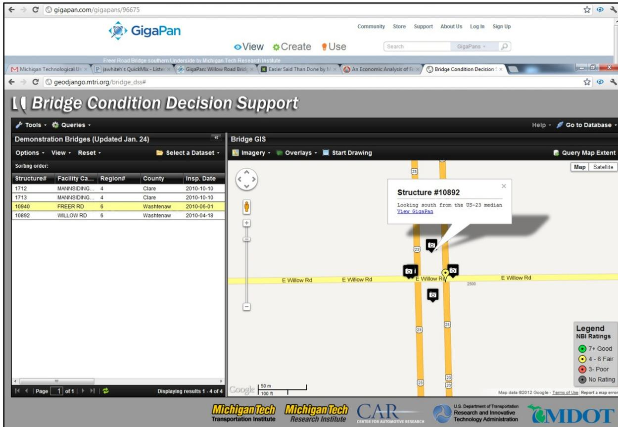
Figure 6-5: An example of the Willow Road bridge GigaPan images being made available through the DSS. The user clicks on the camera icon and is taken to the bridge panorama hosted at [gigapan.com](http://gigapan.com).
