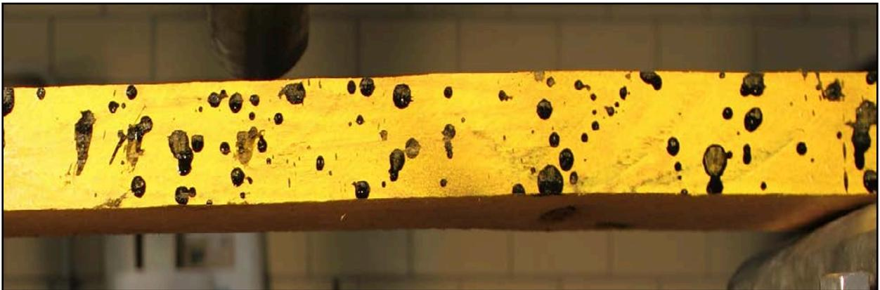
Figure 9-8: Wood Beam with speckle pattern.
