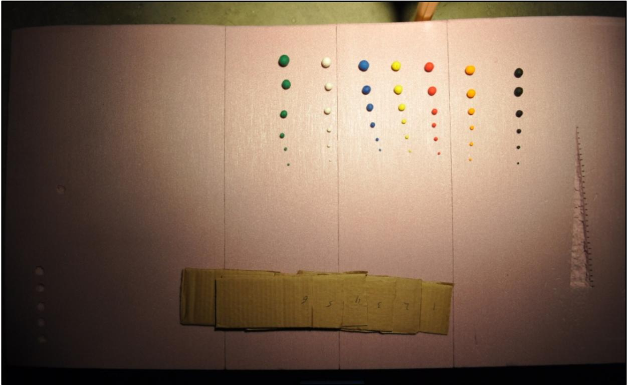
**Figure 4-1:** Photo taken of the foam board used to determine the restrictions of PhotoScan. The light source is directly overhead simulating conditions around noon where the presence of shadows is reduced.
