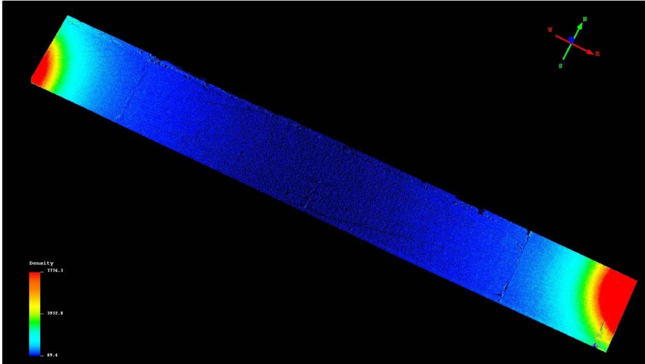
**Figure 7-9: Point cloud density image of Willow Road bridge span over US-23. Note the dramatic fall-off in density of points from ends to center (red to blue, high to low). Features in the blue central areas are unlikely to be able to be resolved successfully.**
