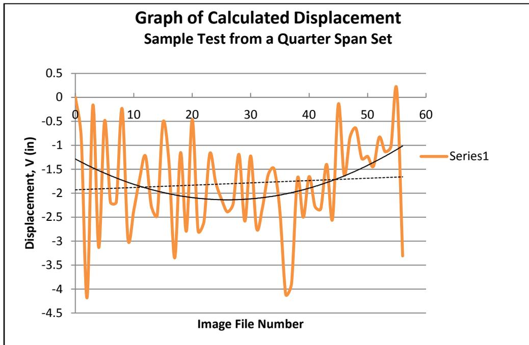
Figure 9-15: VIC-2D plot of calculated displacement for a test series.
