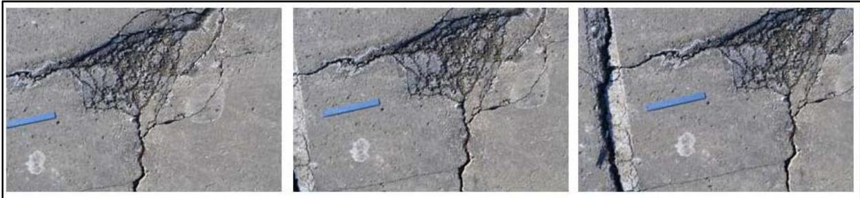
**Figure 4-4: A series of photos that were taken from the parking lot test covering a spill that was used for initial testing with generating area calculations with the DEM outputs. Notice the 60% overlap.**
