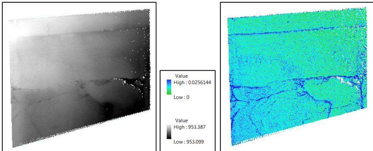
**Figure 7-8: ArcGIS ArcMap Willow Road bridge subset deck DEM displaying point elevation (ft) for a LiDAR subsection displayed as a greyscale DEM (left) and a symbolized raster (right). Bridge deck features such as cracks can easily be seen the symbolized raster LiDAR image at right.**
