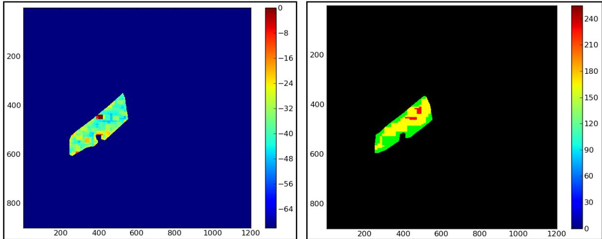
**Figure 11-4: Pixels extracted from Mannsiding Road NB image shown after speckle contrast enhancement with dB color scale (left) and after pixel value classification into a "stoplight" decision support image (right).**
