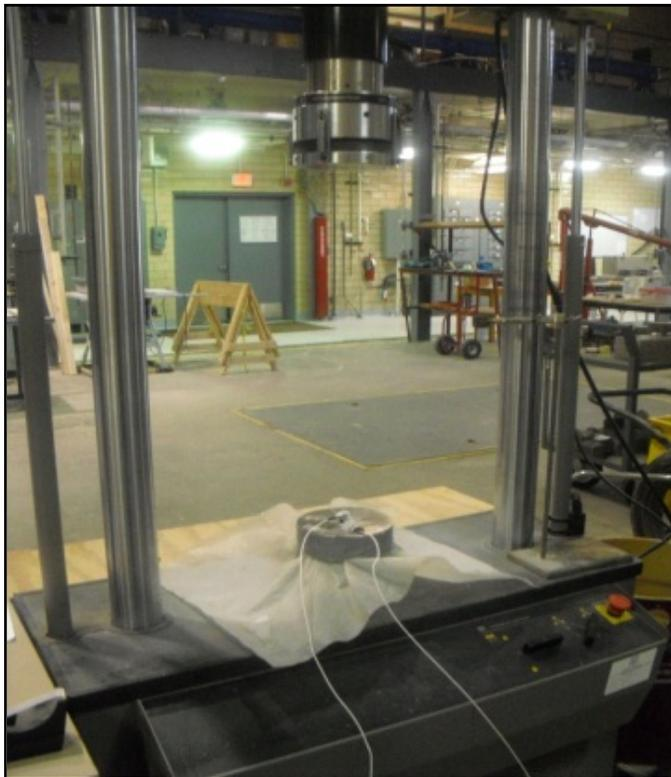
**Figure 9-20: Accelerometers on the 810 Material Test System.**
