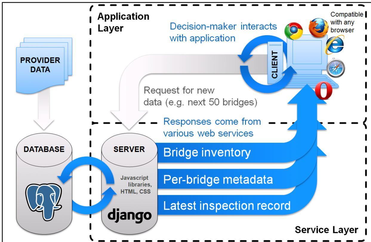
Figure 13-2: Concept diagram illustrating the components of the software architecture in the application and service layers, the location of the client and server within these, and how they communicate with each other.
