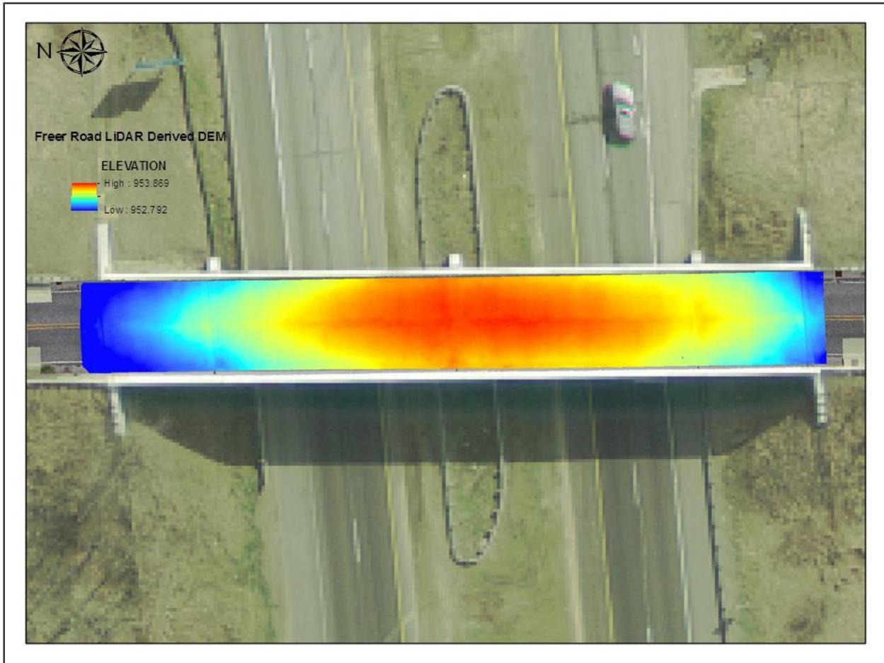
**Figure 7-28: The Freer Road bridge deck DEM over one foot per pixel aerial imagery and the high resolution orthophoto of the Freer Road bridge deck. The DEM is approximately 220 ft long with a spatial resolution of 3 cm per pixel.**
