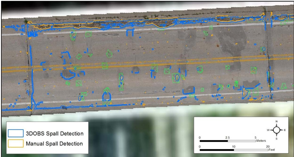
**Figure 4-20: A Willow Road bridge comparison of 3DOBS detected spalls (blue polygons) and manual digitizing of spall locations (orange polygons). The green polygons were painted on to the bridge deck by MDOT personnel and represent delaminated areas as detected by the hammer sounding.**
