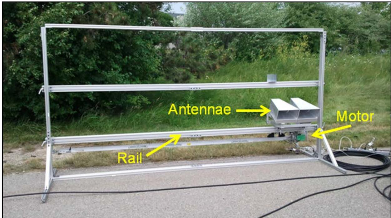
**Figure 10-3: 2D field portable RaDAR translator apparatus.**
