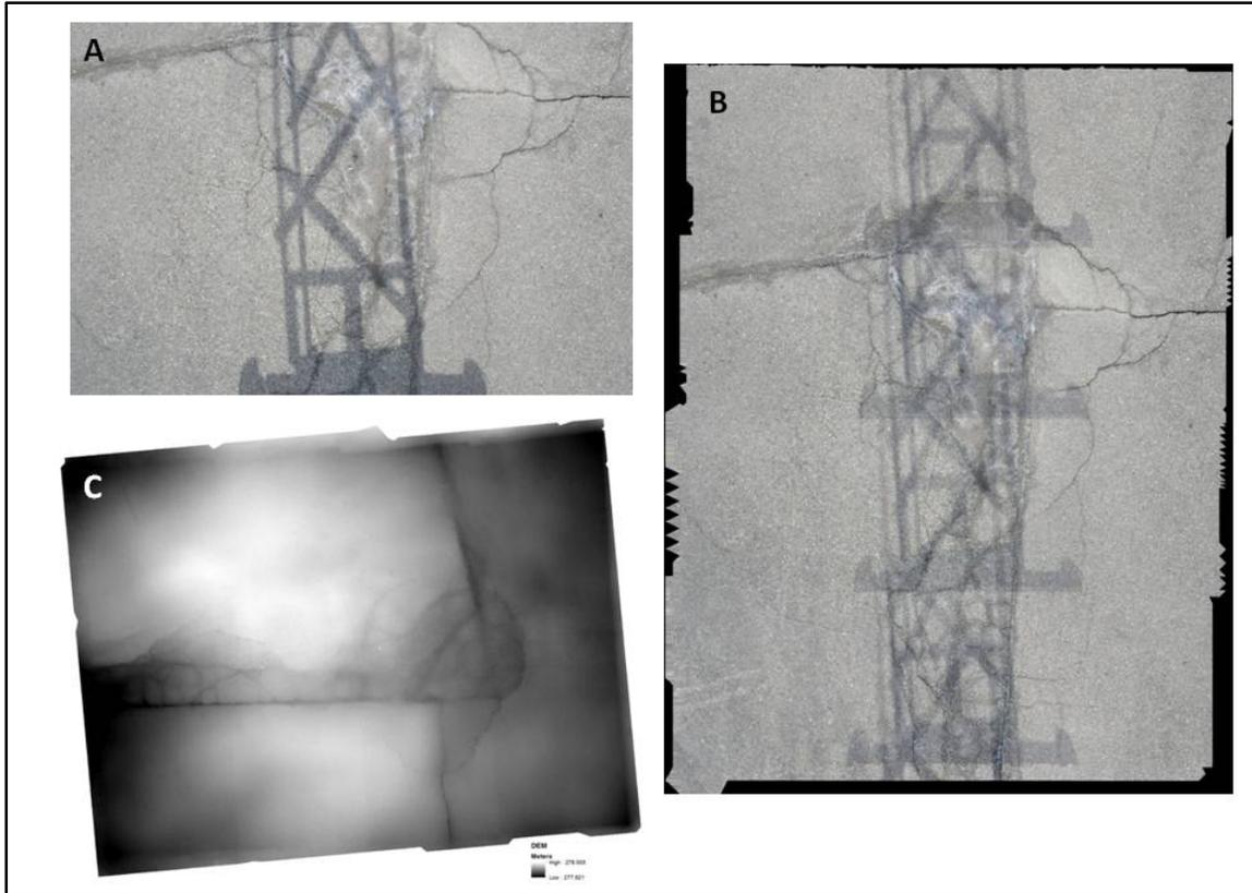
**Figure 4-13: Photos captured by 3DOBS contained the shadow from the vehicle mount as shown in A. Despite the shadow PhotoScan was able to align the photos (B) and generate an accurate DEM (C) of the parking lot surface.**
