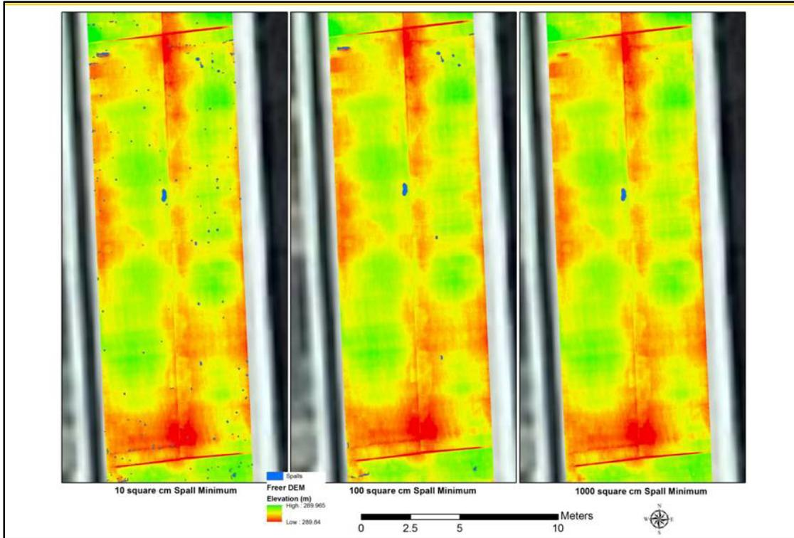
Figure 4-8: Differences in minimum spall sizes as from the spall detection algorithm. Starting on left, the images depict spalls larger than 10 cm<sup>2</sup>, 100 cm<sup>2</sup>, 1,000 cm<sup>2</sup> respectively. Data from Freer Road bridge.
