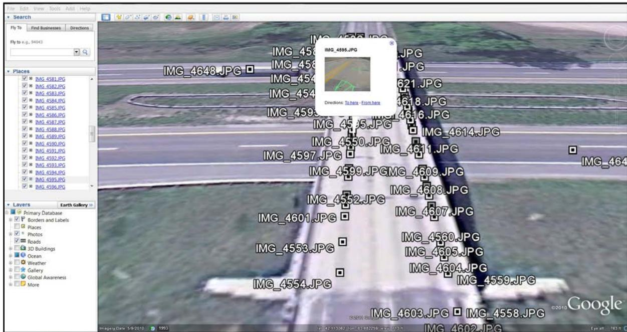
**Figure 5-5:** Example of the location of the digital photographs being displayed in Google Earth; each box contains a hyperlink to a full-resolution view of the photo taken at that location.
