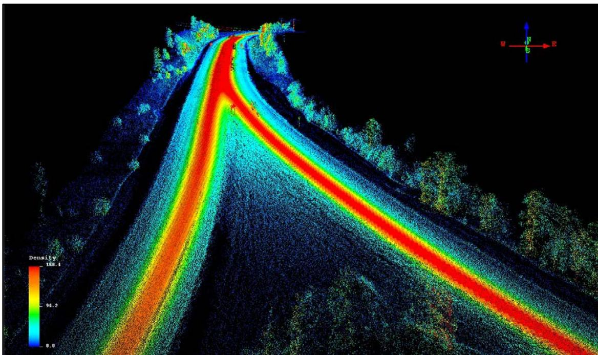
**Figure 7-26:** An example of the point cloud density decreasing from scanning-vehicle /scanner-centerline. Image shows US-23 NB (left) I-96 (right) merging. Vehicle speeds; ~45 mph (US-23) and ~35 mph (I-96).
