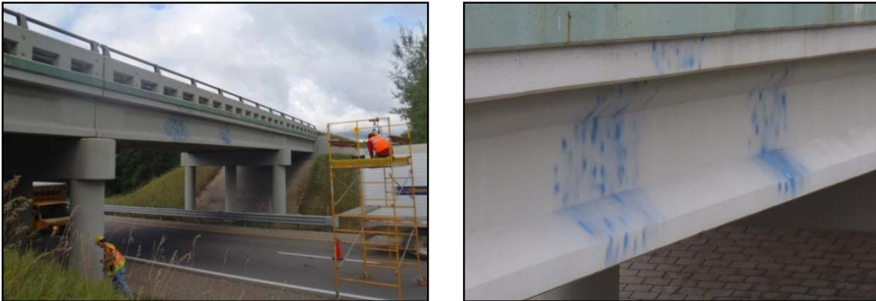
Figure 9-12: DIC setup at Mannsiding Road bridge and detail of girder with speckle patterns.
