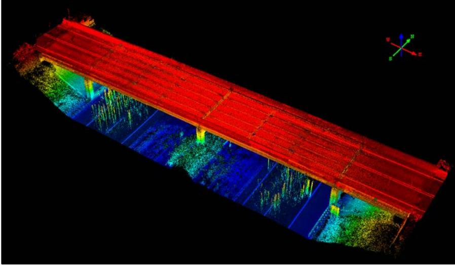
**Figure 7-6: An example of geo-registered, geo-referenced LiDAR point cloud of the Willow Road as collected by MDOT. Point elevation (color) and intensity are displayed. This LiDAR point cloud contains more than 186 million points. Quick Terrain Modeler software was used to generate the point clouds and DEMs.**
