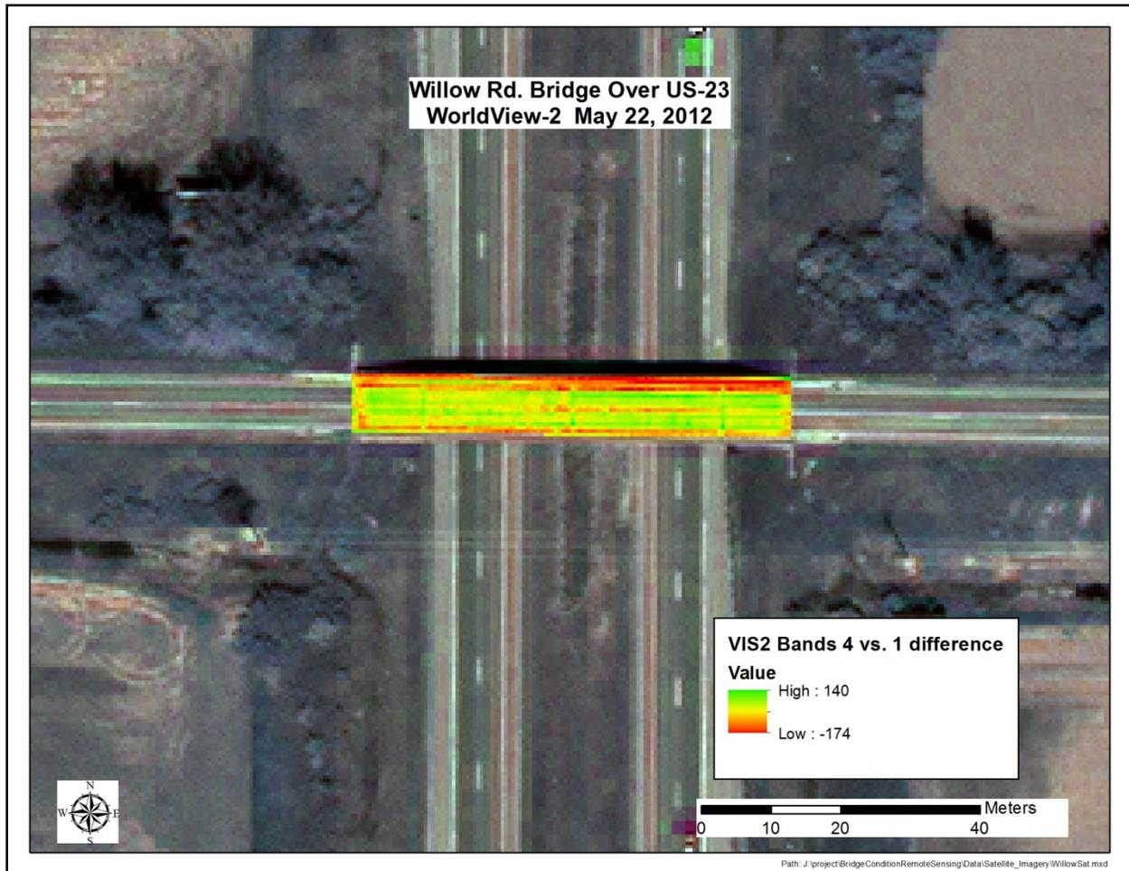
**Figure 12-2: The VIS2 calculation displayed in color for the Willow Road bridge using WorldView-2 commercial high-resolution satellite imagery. Red and green areas (relatively low and high values) show high contrast between the blue and infrared spectral band information.**
