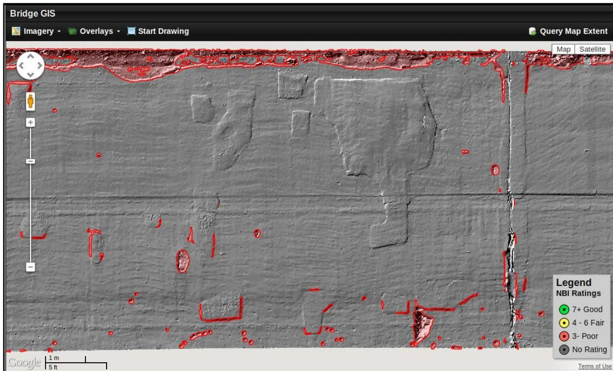
**Figure 13-10:** Screenshot from the DSS of the hillshade DEM layer for the Willow Road bridge with spalls outlined in red; note that bridge joints have been removed from the spalls layer and that the vertical accuracy is so fine that patches are clearly seen.
