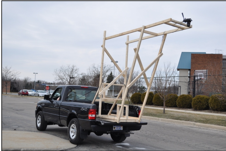
Figure 7a: Demonstration of close-range photogrammetry image collection system for bridge deck surface condition evaluation, currently undergoing further testing.
