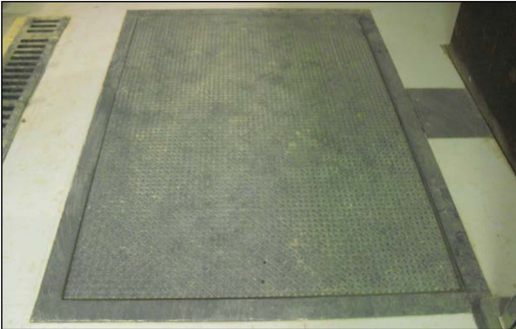
Figure 30: Floor scale loading platform used to simulate scaffolding movement.
