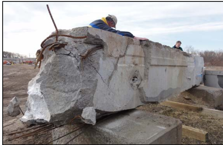
Figure 1e: Silverbell bridge box-beam saved for radar sensing work by the Oakland County Road Commission after the bridge was recently removed from service due to poor beam condition.
