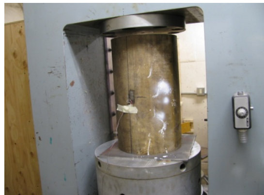
Figures 1c & 2c: Bridge pylons on a pallet and pylon before a compression test.
