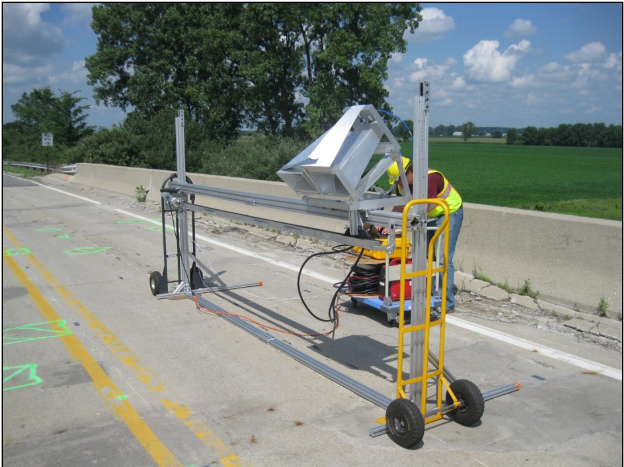
Figure 46: More "mobile" translator apparatus and radar equipment. It is easy to view how such a system could be adapted for use on a moving vehicle.
