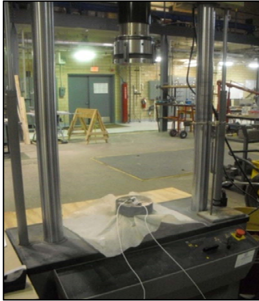
Figure 11: Accelerometers on MTS testing machine.
