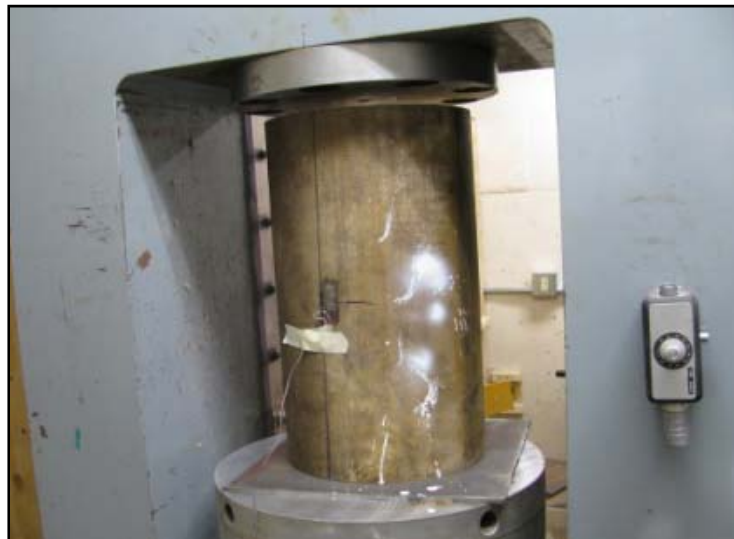
Figure 1d: Section of a bridge pylon (concrete-filled pipe) in load frame compression test.
