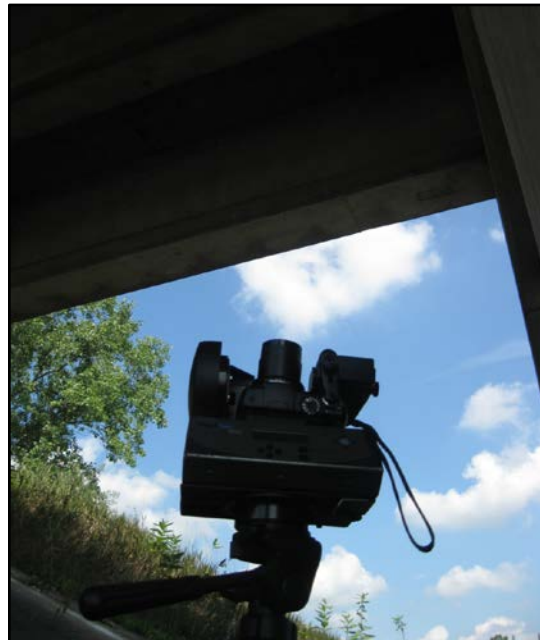
Figure 15: An example of the GigaPan being used to collect high-resolution bridge inventory photos during August, 2011 field demonstrations at Willow Road bridge.
