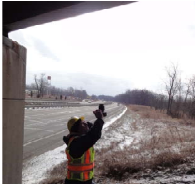
Figures 5a & 6a: Researcher taking photos of the underside of 6 Mile Bridge at US-23 near Brighton, MI. The distance from the camera to the spalls was approximately 2.5 meters (8 feet). Photo taken of spall on deck bottom surface from the field test shown above at 6 Mile/US-23 Bridge.
