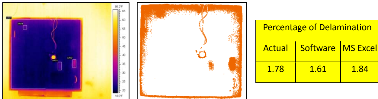
Figures 4c & 5c / Table 1c: Results of calculating the percentage of delaminated areas on the concrete slab using three different methods.
