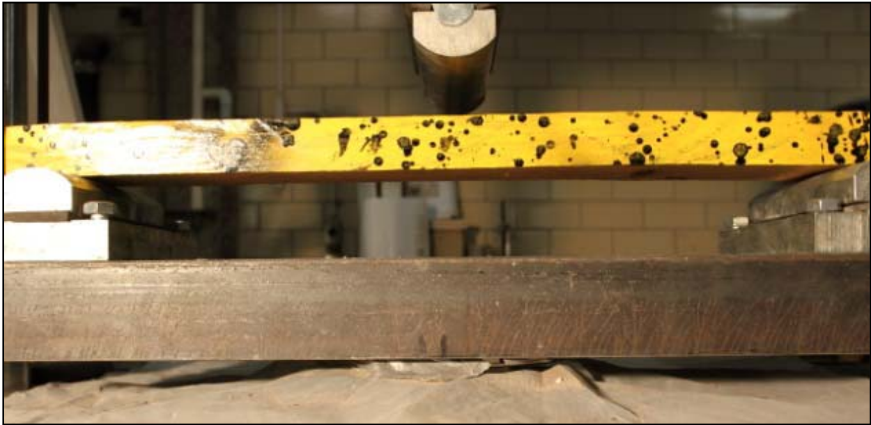
Figure 6d: Picture of “two-by-four” wood specimen in testing machine.
