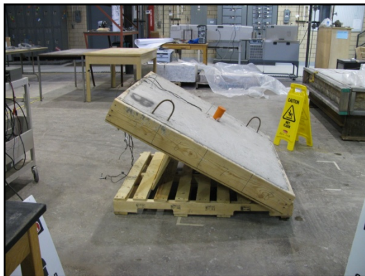
Figures 4c & 5c: ThIR lab test set up showing camera and slab perpendicular to each other.
