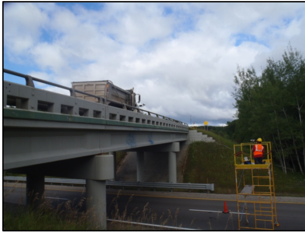
Figures 25 & 26: Load truck going over bridge and close-up of camera and tripod setup on scaffolding.
