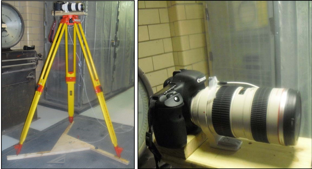
Figures 14 & 15: Camera on stable tripod and detailed of mounted accelerometer.
