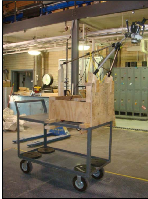
Figure 15: FLIR SC640 ThIR camera mounted on the cart for field demo.
