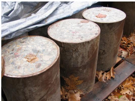
Figures 1c & 2c: Bridge pylons on a pallet and pylon before a compression test.
