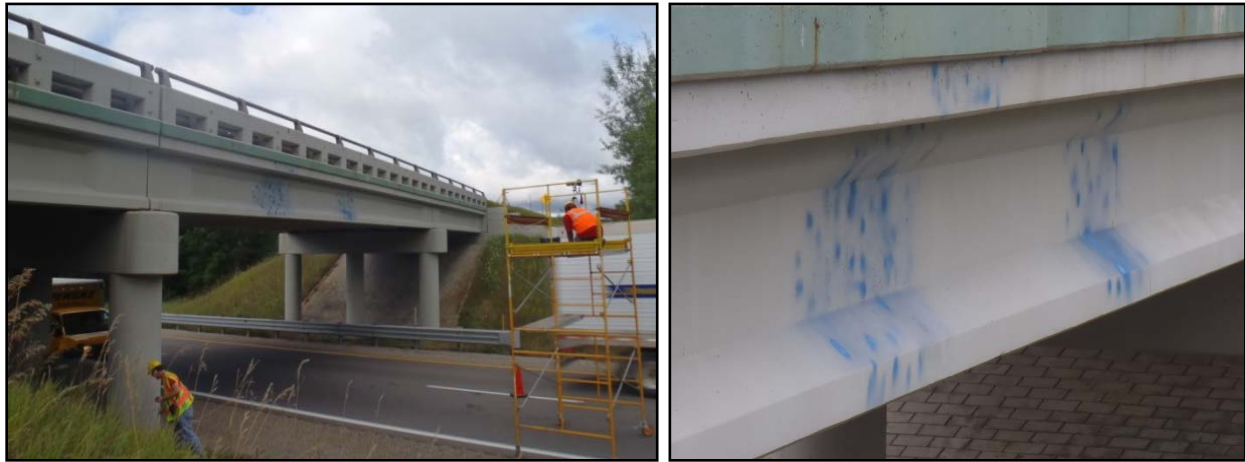
Figures 23 & 24: DIC setup at Mannsiding Road bridge and detail of girder with speckle patterns.
