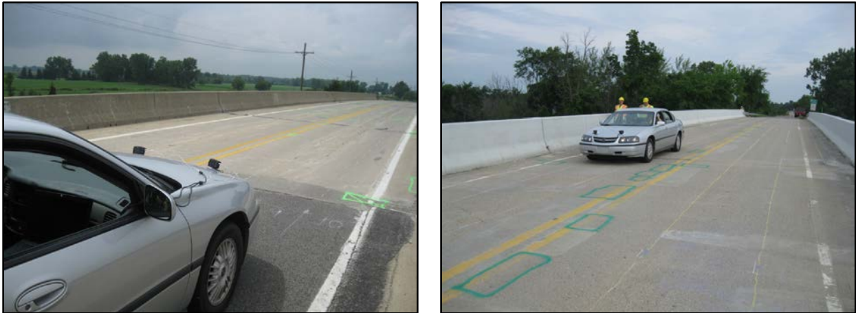
Figures 9 & 10: The BVRCS being deployed on Freer Road bridge to capture a photo inventory.
