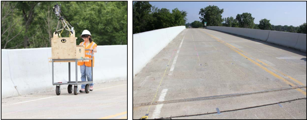
Figures 17 & 18: ThIR camera mounted on the cart with “homemade tripod” system and chalk and duct tape grid layout on Freer Road bridge.
