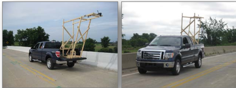
Figure 1: 3DOBS deployed for data collection from the back of a moving truck
