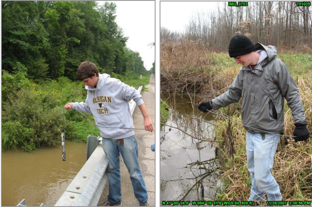
Figure 3-1: Two examples of the Horiba U-22XD instrument being used by MTRI interns to collect water quality data in the Tiffin River study area. The photo in the left shows the instrument about to collect data in a turbid segment of Bean Creek; the photo on the right shows the instrument being used to actively collect data along part of Lime Creek
