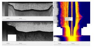
Down looking (50 and 200 kHz) capabilities vegetation discrimination; SSS provide is provided at 455 or 800 kHz to map up to 250 feet either side of the vessel.
