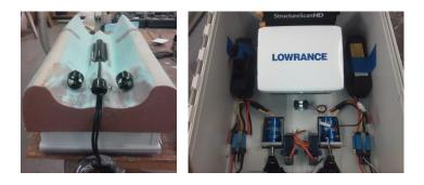
BathyBoat collects sonar data using a Lowrance HDS Sector Scan System. This allows for down looking (50 and 200 kHz) Side Scan Sonar with data recording and GPS in a single unit. This is combined with an internal GPS which collects a positions at 5Hz. This sonar allows for a high density of points to be collected as it can store up to 12,000 points internally. Bathyboat can be customized to use other sonar systems.
