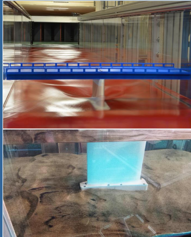
Live Bed Bridge Scour Experiments
