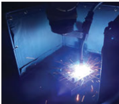
MIG welding robot printing a steel part (Photo Credit: Mike Groeneveld)
