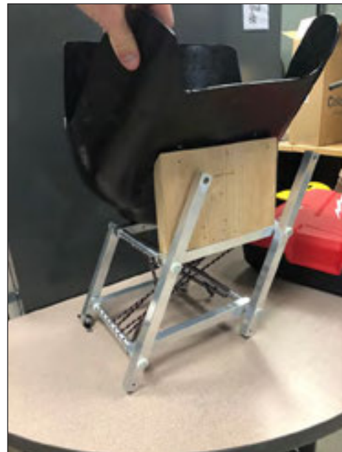
Prototype of the team's parallelogram-frame sit ski (Photo Credit: Joseph Vann Linn)
