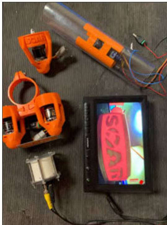
Components of the replacement ROVs designed and produced by SOAR
