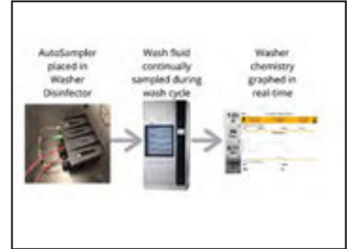
Schematic of the intended AutoSampler process: continually collecting samples then outputting real-time data
