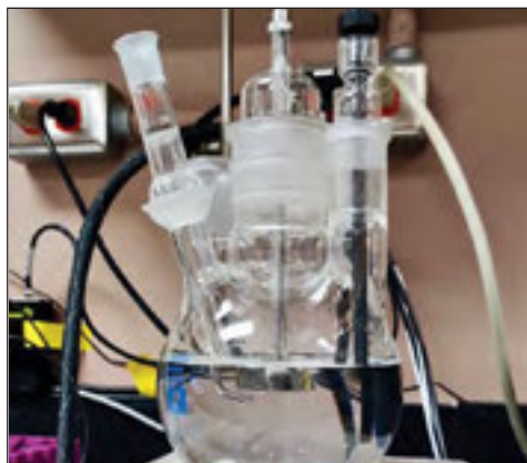
EIS accelerated corrosion testing (Photo Credit: Henry Vandermark)
