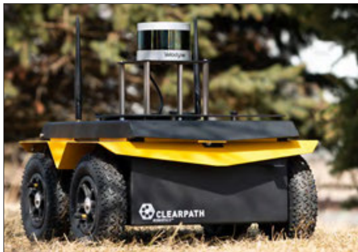
A Clearpath Jackal with a mounted lidar (Photo Credit: Clearpath)
