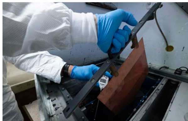
Students make circuit boards by selectively etching away copper to leave traces that connect components.
