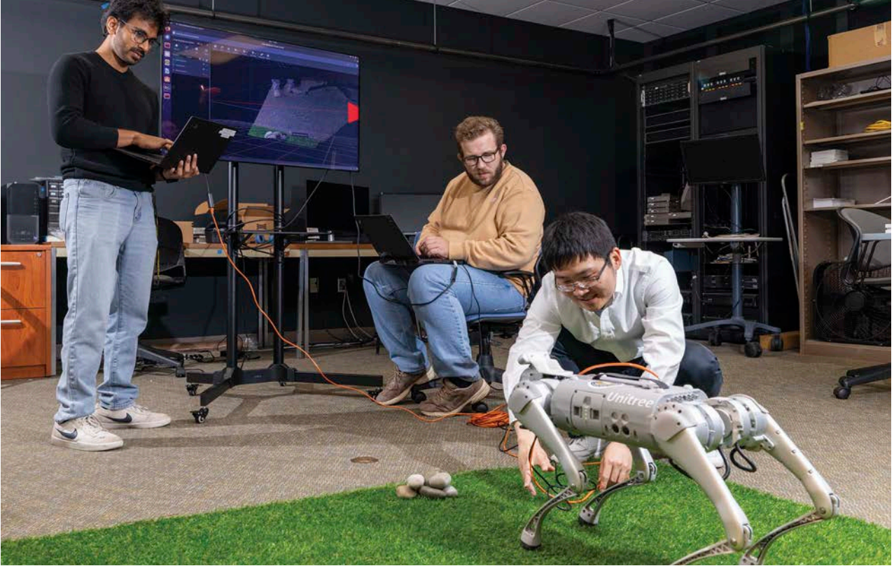
Evaluating terrain classification and adaptive gait-switching algorithms on a legged robot. (L-R: Shivayogi Akki, Anders Smitterberg, Tan Chen)
