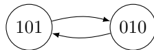
(a) Legitimacy graph for predicate L_i(x_{li}, x_i, x_{ri}) \stackrel{\text{def}}{=} ((x_i \neq x_{li}) \wedge (x_i \neq x_{ri})) where each x_i \in \mathbb{Z}_2 .
