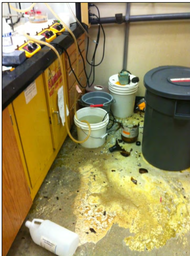
Figure 9.2 – Container Failure Due to Mixing Incompatible Waste Streams
