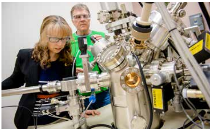
Assistant Professor Kathryn A. Perrine and ACMAL Director, Owen Mills, transfer a sample into the new XPS instrument for surface analysis.
