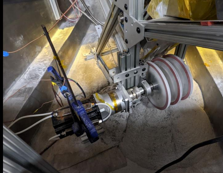
Vacuum Rated Direct Shear Test
