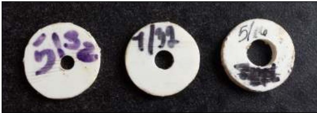
Figure 5: Flow-reducing discs
