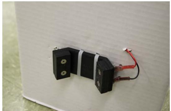
Fig. 2. Female magnetic connector
