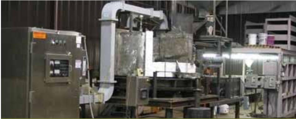
Pictured above is a hybrid furnace used as part of an energy-efficient method for making steel, with synthetic gas as a byproduct.
