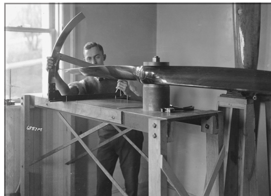
At FPL's propeller laboratory, effects of changes in humidity and temperature were carefully measured and recorded.
