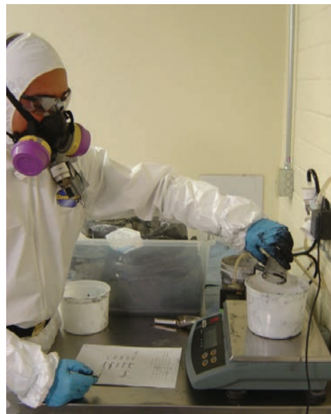
Figure 7. Weighing of carbon nanotubes.
