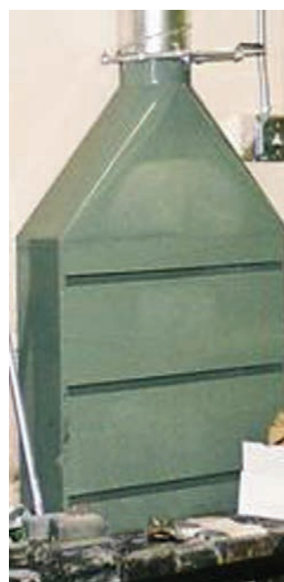
Figure 9. Exterior hood (note that the work area is in front of the hood entrance)
