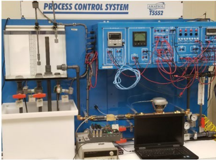
Figure 8 (b): SoT and ECE PLC Lab – Process Control Systems
